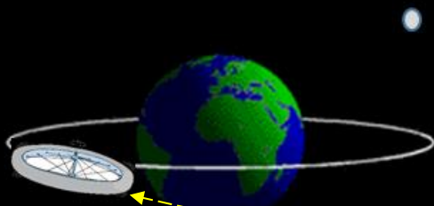
Its geostationary orbit is at 22,000 miles above the Earth's surface
